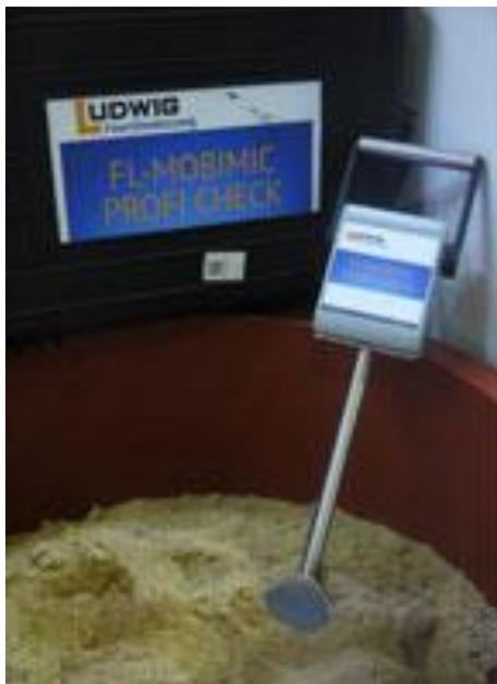
This testing device is used to accurately determine the moisture content and temperature of a specific aggregate before batching, during the mixing cycle and after discharge of the mixed concrete. Key to the device's versatility is that it can be used in several places during the mixing-and-batching process.
