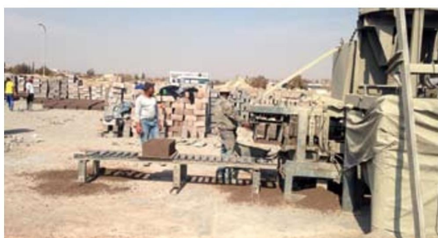
This UNI Plant brick making machine has been in service at Leo Bricks for six years and is still running well – producing 3 000 hollow block bricks per shift every day
