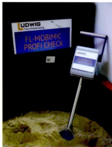
(Above, from top): Manfred Ludwig, MD of Ludwig Moisture Control; the new FL-Mobi Mic Profi-Check aggregate moisture testing device.
