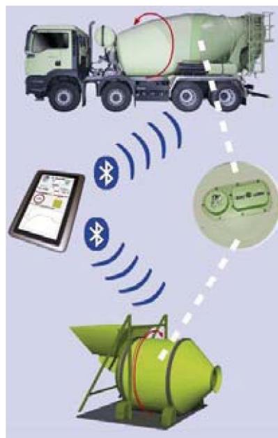
FIGURE 1 FL-MOBI MIC. Wireless moisture monitoring
