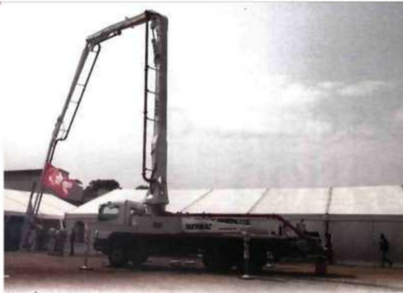
The impressive Sermac pump extends 36 m in height
