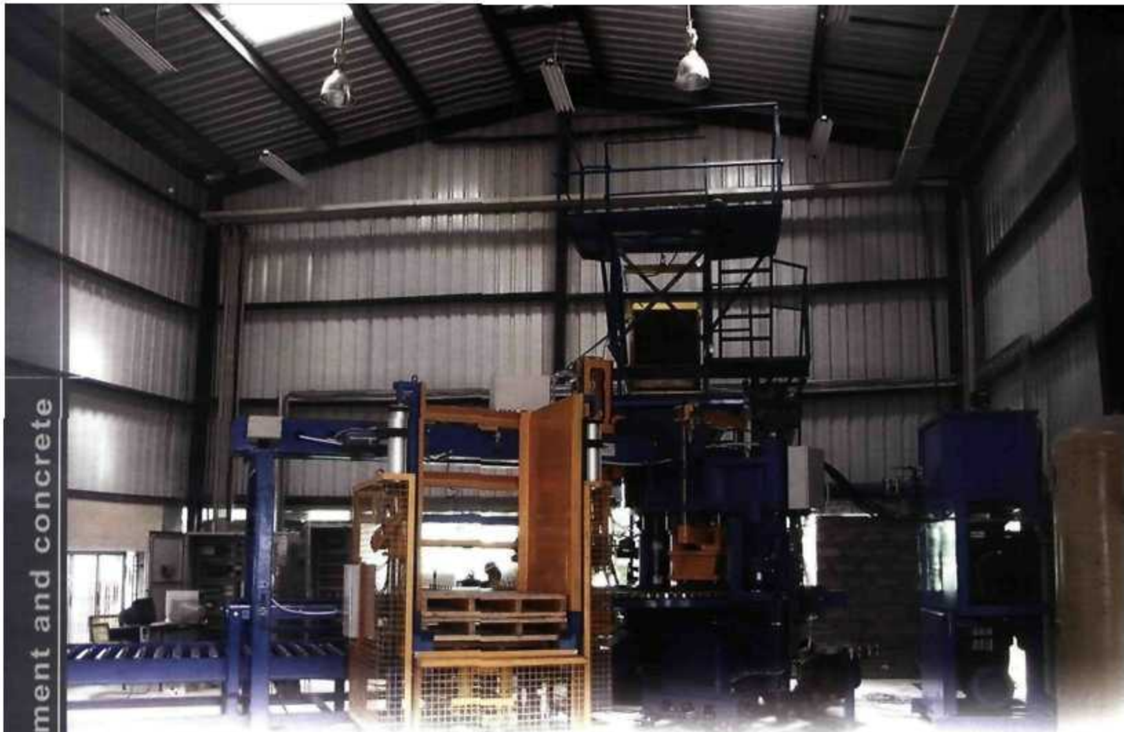
A customer installation of a three-stage press with take-off, showing a complete press installation
