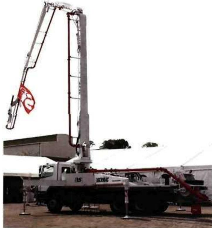
**Above:** Ikhaya Technologies' i-brick. **Right:** Sermac offers a complete range of concrete pumps with booms from 21-65 m, together with several fold configurations.
