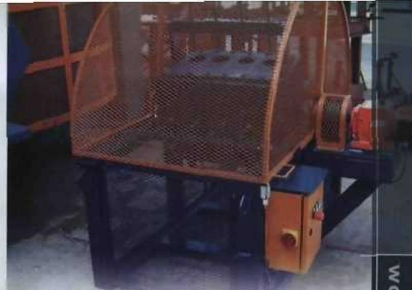
*The abrasion testing machine is a square-shaped drum, onto which four pavers can be bolted to each face of the machine*
