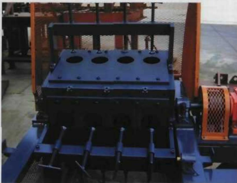
Pan Mixers South Africa (PMSA), in partnership with the Concrete Manufacturers Association (CMA), has manufactured a robust abrasion testing machine to assist customers in complying with the revised South African Bureau of Standards (SABS) abrasion requirements for concrete pavers.
