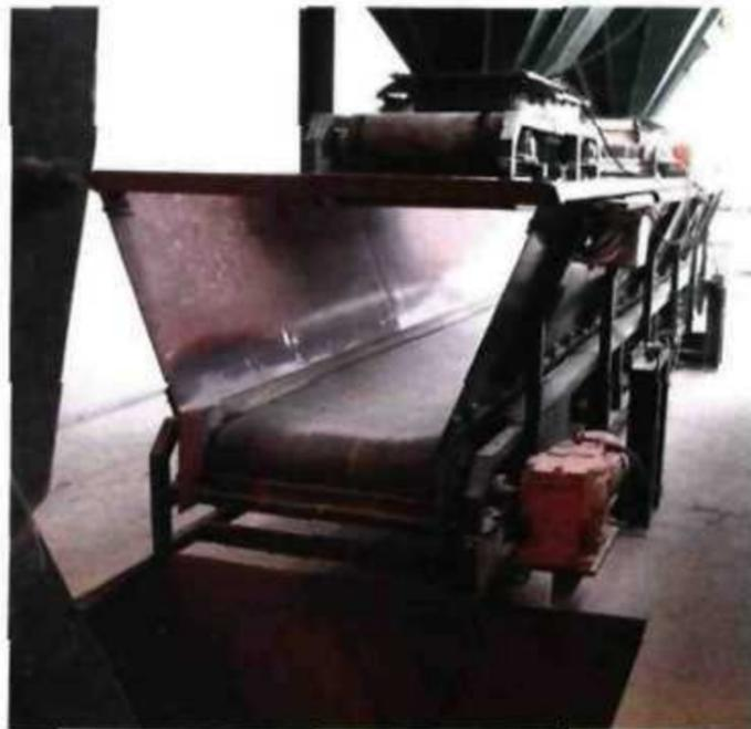
PMSA extractor conveyors extract aggregates from the bins and deposit them onto the weigh-scale conveyor. The key stage at the start of any concrete process is to accurately weigh each aggregate so as to achieve consistent batches of concrete.
