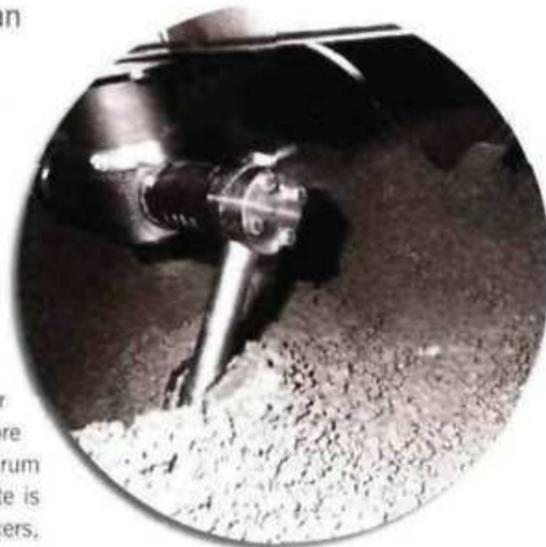
The mixing action of a planetary pan mixer. The whole pan is rotating in one direction while the arm is rotated in the opposite direction. Pan mixers mix very intensively because material is being continually chopped and split in all three dimensions as it is repeatedly fed from the centre to the outside of the mixer.
