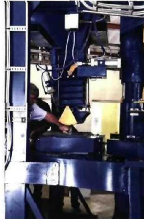
A 400 t press is used on a three-station revolving turntable to remove the water from the wet concrete.
