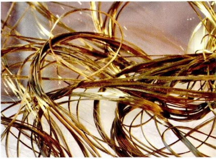
StoneRod, made from basalt rock.
