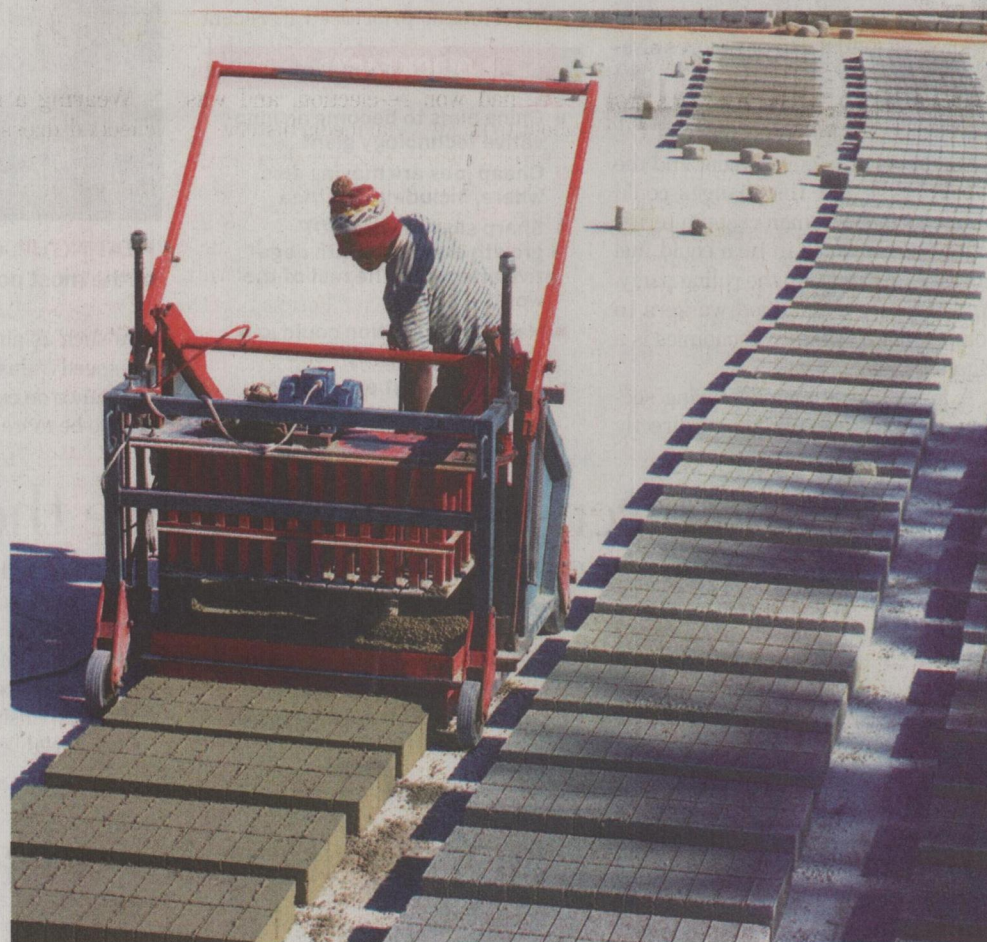
CONSTRUCTION SCHEMES: A brick maker lays out a fresh batch of bricks from a quality machine available under the scheme to create long-term employment. PICTURE: GALLO IMAGES
