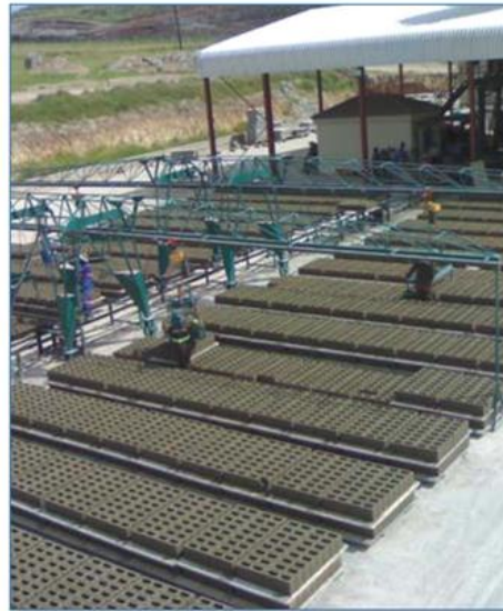
Laman owns two VB4-X machines, which are used to convert aggregate into M140 concrete blocks for the low-cost housing market.
