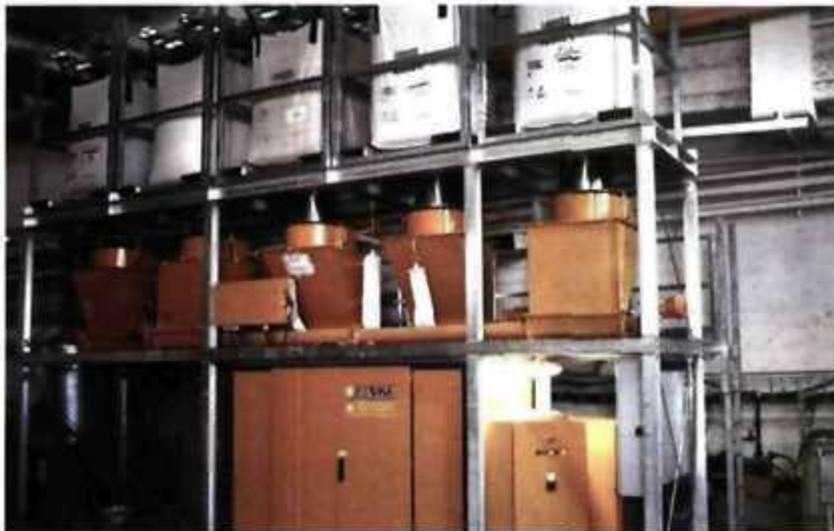
station for dust-free connection. "The level of pigment within the bags is continuously-monitored and displayed on the control panel of the unit - to enable the production operator to determine when a new bag of pigment will be required, and to avoid any disruption to production," adds Ebeling.
