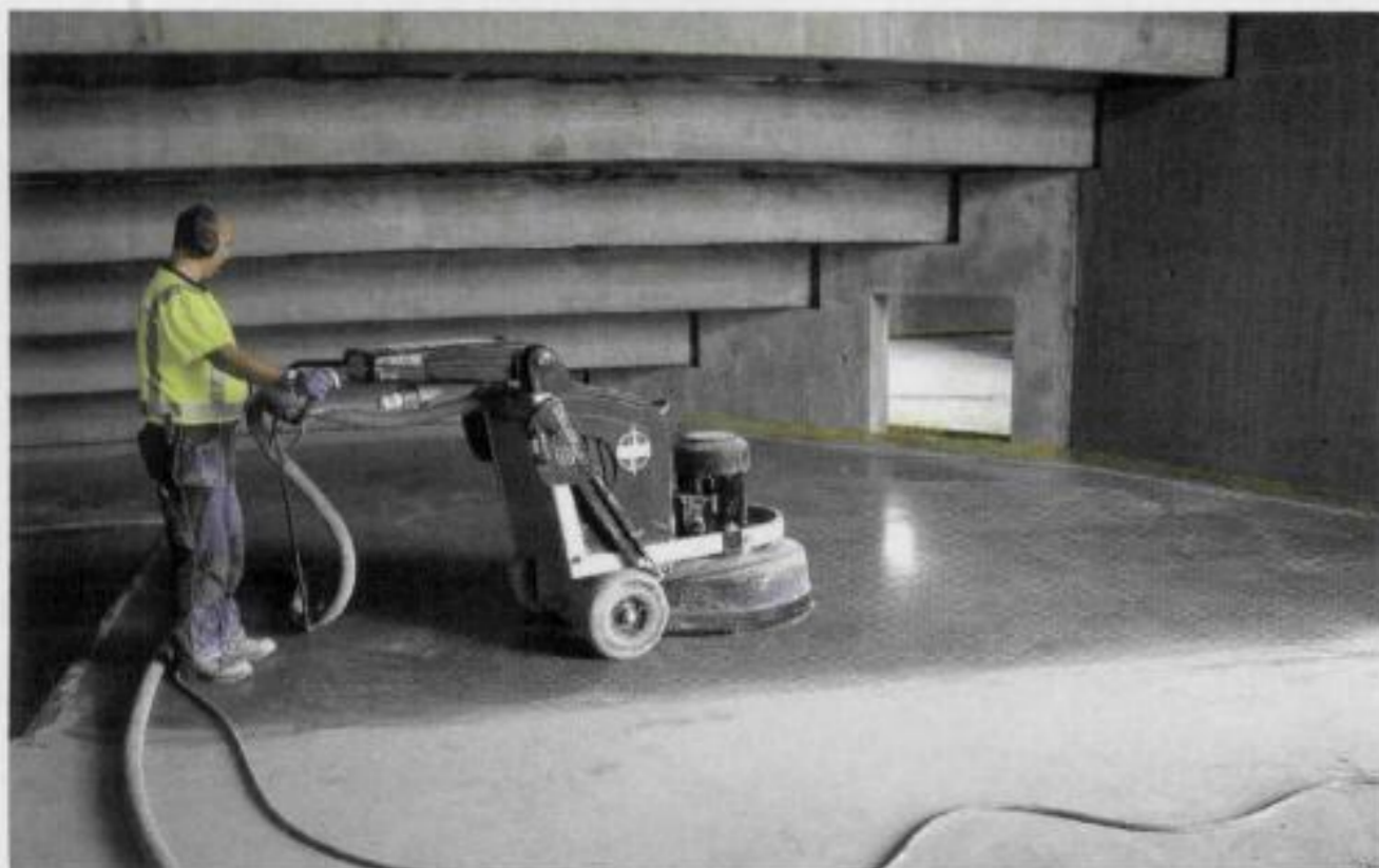
The HTC 800 HDX is fitted with a powerful 15 kW motor, and is ideal for high demands on cutting capacity, as it comes with 55 kg of additional integrated weights
