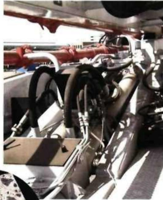
**Above:** The Sermac concrete pump uses two hydraulically driven pistons to pump the concrete through two cylinders. When the pumping piston reaches full stroke, the pulling and pushing reverses and an S-valve moves across to the full cylinder's outlet to give continuous concrete flow. **Left:** HTC concrete grinding equipment can grind and polish concrete so that it looks like marble.
