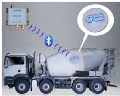
Ready-mix truck with a receiver module (above) and below, ready-mix truck with an external receiver.
