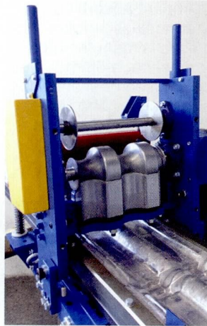
PMSA's quick maintenance on SPS712 with tilt-up extrusion box.
