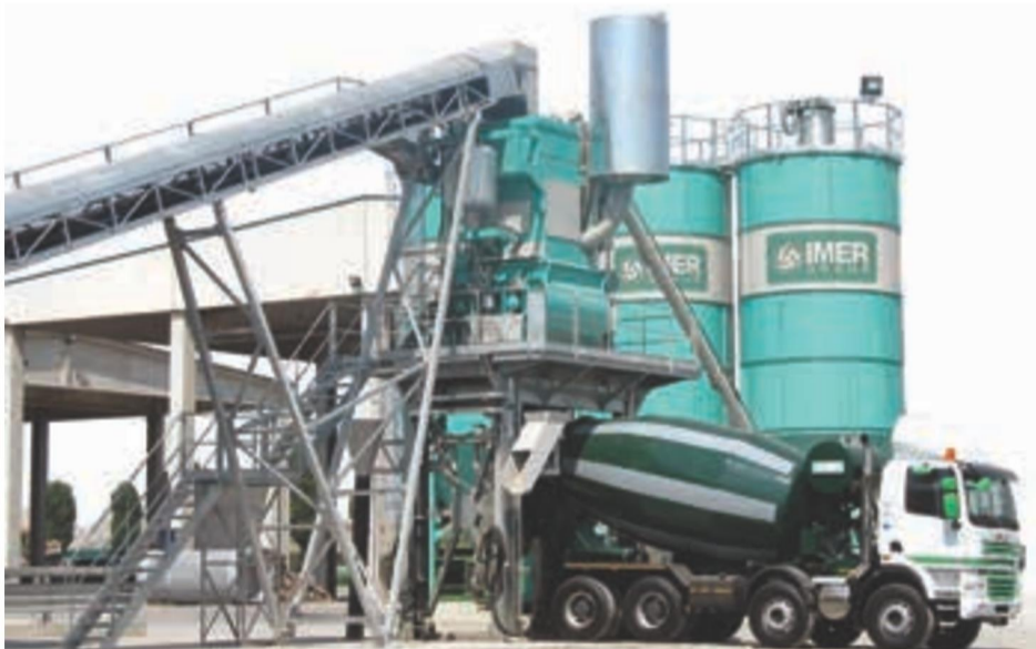
Automated IMER wet batch plants, now available in South Africa from Pan Mixers, create fully mixed concrete, which ultimately reduces costs, as it eliminates the need for high-speed mixing in the truck prior to dispatch.
