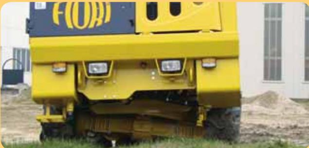
Great stability, even at full load, these machines are also on off-road routes difficult due to the front swinging axle. Extremely compact machine for use in confined spaces.
