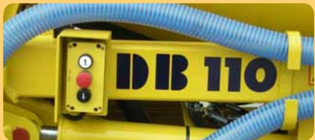
Additional device the operator can also rotate the drum from the ground and in addition to the cabin. The device is located near the discharge chute to better control the speed of discharge of concrete.
