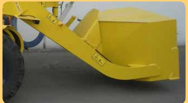
Even though small, the model DB 110 offers a high standard of the equipment designed to assist the operator. Is equipped as standard with the automatic shutter of the mechanical loading shovel to avoid loss of materials in the loading phase inside the drum.
