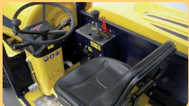
With open ROPS cab. With the driving reversible 180 ° for better visibility during the loading of materials. It can be equipped with trilateral glass or closed cab with heating.
