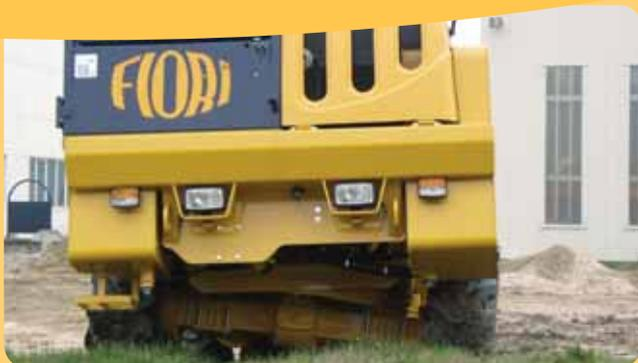
Great stability, even at full load, these machines are also on off-road routes difficult due to the front swinging axle.
