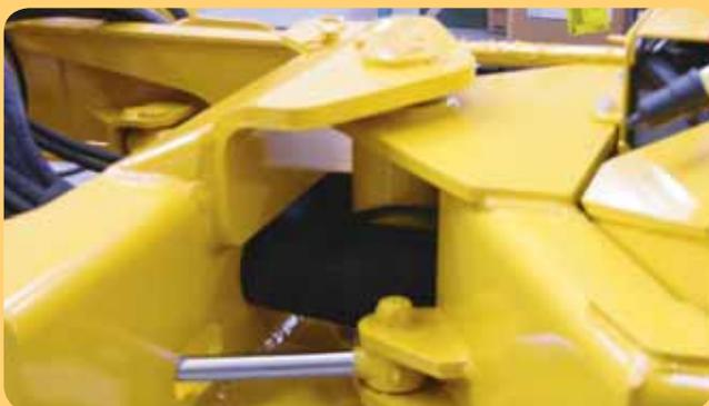
High-tensile electrowelded steel frame, articulated with frontal oscillating bridge for greater stability, and double soft-system jack for faster and comfortable handling.
