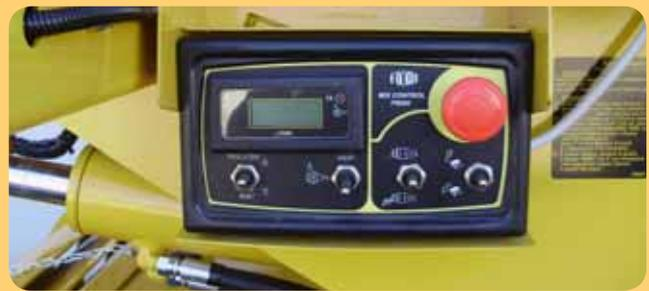
Unique in its class with MIX CONTROL device . Digital flowmeter programming the quantity of water in the concrete, for the start / stop of the water pump and for the rotation of the drum. All in one small panel near the discharge chute . The same operations can be done from the cab.
