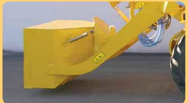
Even though small, the model DB 180 offers a high standard of the equipment designed to assist the operator. It is equipped as standard with the automatic closing of the mechanical loading shovel to avoid loss of materials in the loading phase inside the drum.
