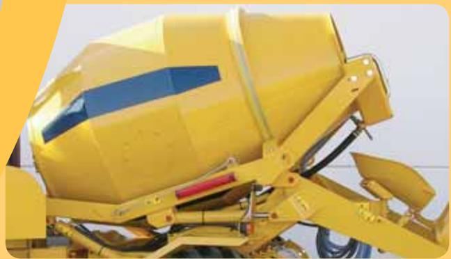
Mixing system tested and approved for the production of high quality concrete due to the particular shape of the drum and the proper system in loading components.
